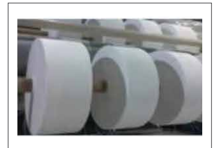
3- Cut off the edges on both sides, eventually become a non woven coiled material.
